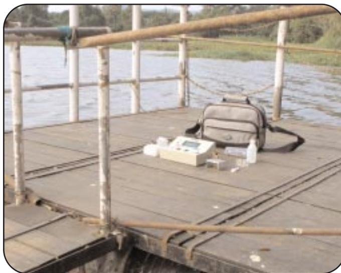
reads out the measured concentrations. The sensor-cartridge is screen-printed, low-cost and can be easily replaced.
