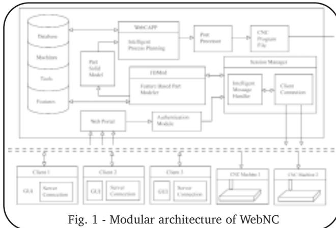
Fig. 1 - Modular architecture of WebNC
