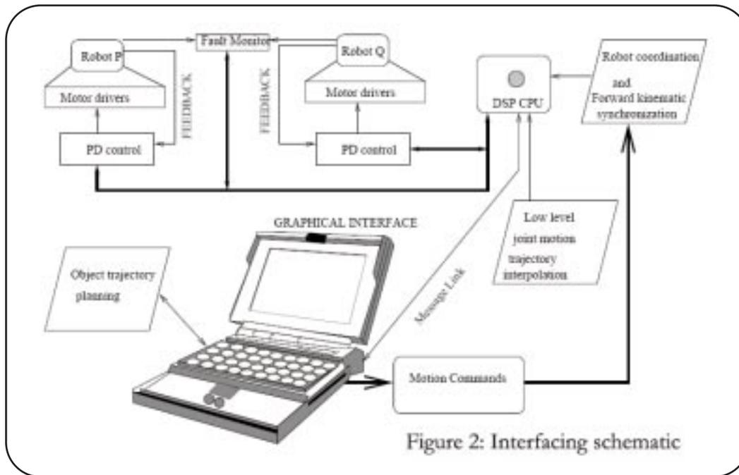
Figure 2: Interfacing schematic
