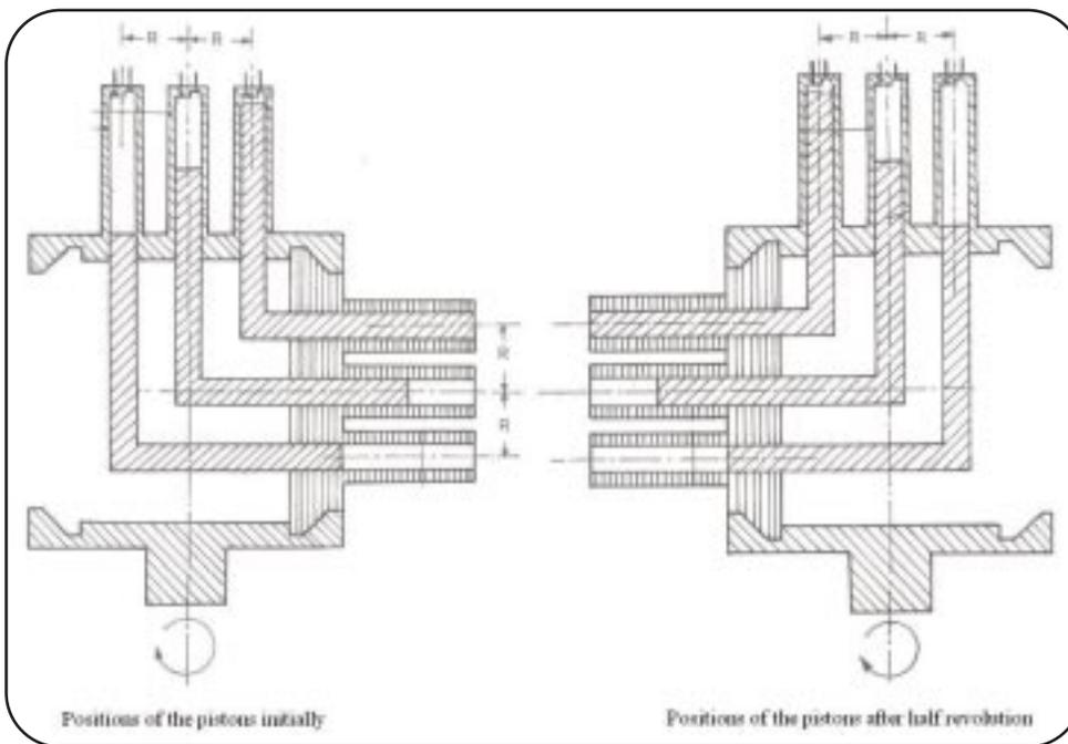
An Indian Patent titled "A compact drive mechanism of a reciprocating machine" was granted to IIT Bombay on 5 June 2006. According to the inventor, Prof S L Bapat, Department of Mechanical Engineering, the objective of the invention is to provide a compact and efficient drive mechanism for a reciprocating machine that is free from side thrust.
