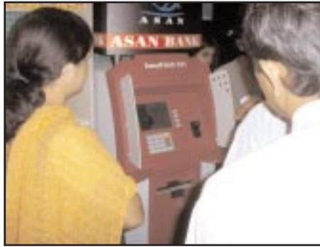
The attractive new design incorporating elements from traditional Indian architecture departs from the current neutral appearance of ATMs. Banks may further customize it to a limited degree. The small size makes it suitable for deployment in places with space constraints. ASAN's ergonomic design suits the typical Indian body dimensions with respect to the height of the keypad and the inclination of the screen. Additionally, the machine has a provision
