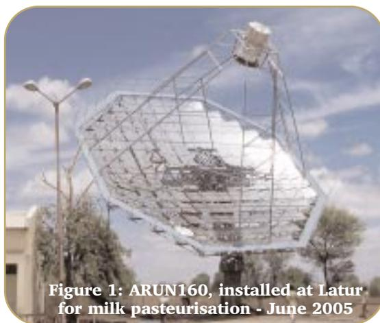
**Figure 1: ARUN160, installed at Latur for milk pasteurisation - June 2005**
