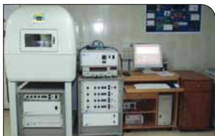
NanoIndenter: a depth-sensor for thin films and small structures
