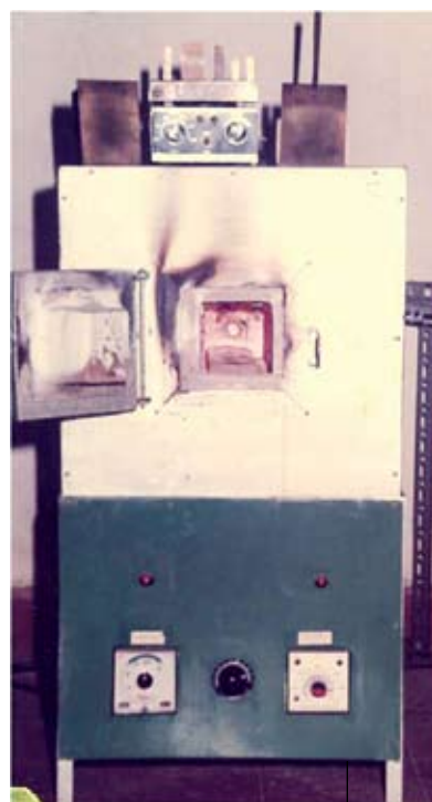
Operating system including mould bars, furnace and hot press
