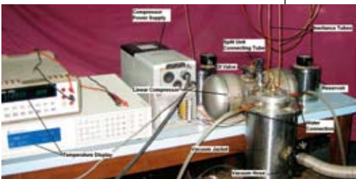
Experimental set up for two stage cryocoolers
