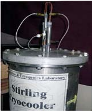
Alpha Stirling cryo-cooler developed using the drive mechanism
