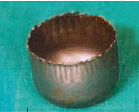
Formation of cup using ANN suggested material specification
