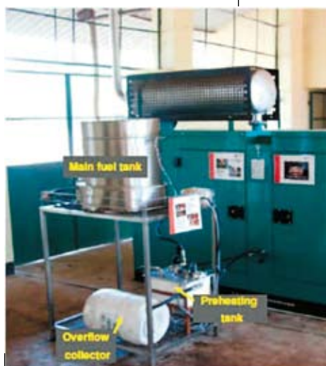
The fuel processor with engine set at Kohla village, Orissa for rural electrification
