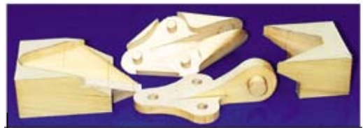
Bracket made on an LOM machine after pre-processing using OptiLOM
