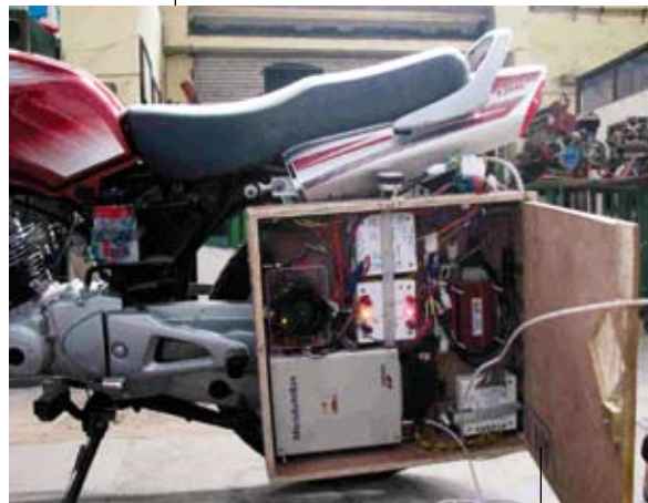
Engine management system fitted on a two-wheeler vehicle
