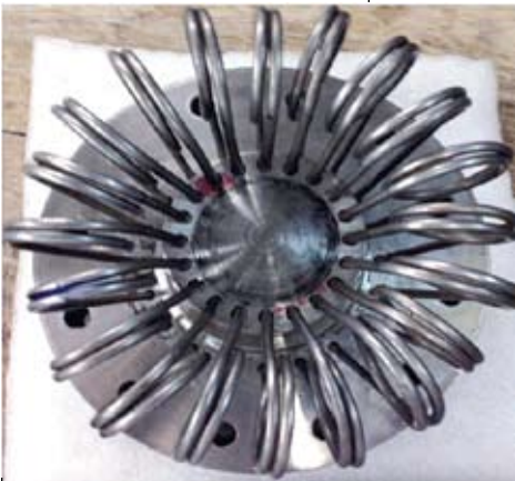
Cylinder Head heat input tubes as modified
