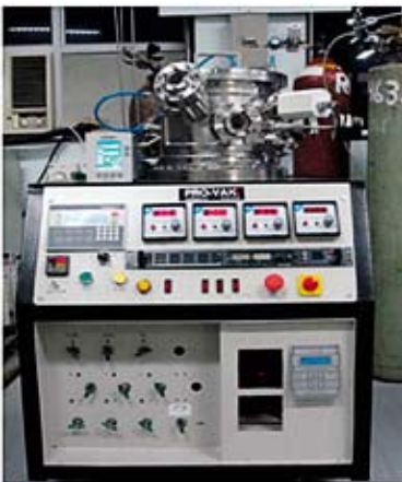
Hot wire processing chamber for treating low k films
