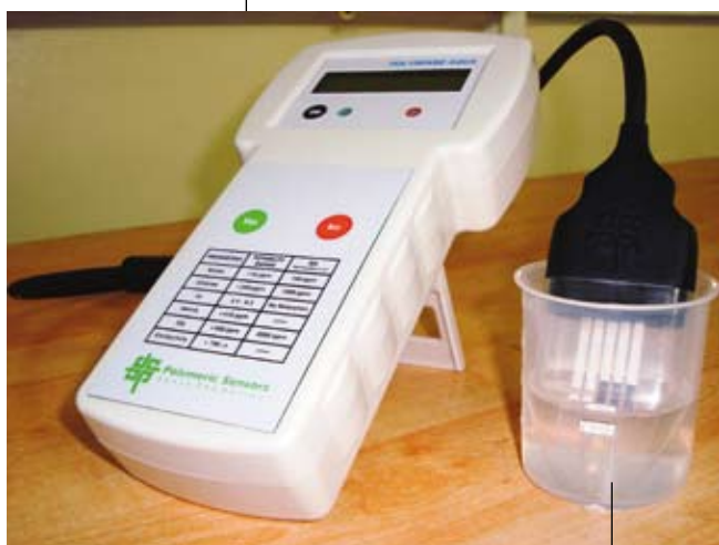
Polysensor used for determination of water quality
