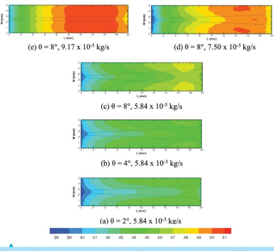
Experimentally measured temperature contours using an IR camera in the proposed microdevice. The figure shows that the uniformity in temperature improves with tuning of the parameters (divergence angle and flow rate).
