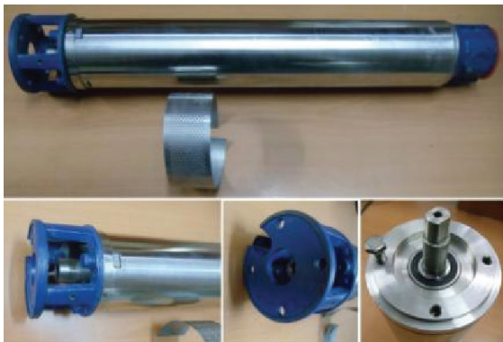
Submersible pump and pump side coupling of the fabricated BLDC motor
