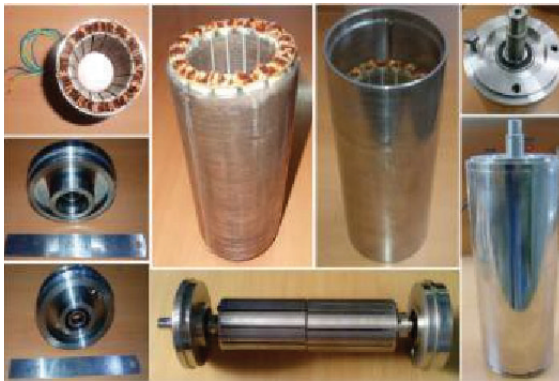
Stator, rotor, end-flanges and the fabricated ferrite magnet based spoke-type submersible BLDC motor
