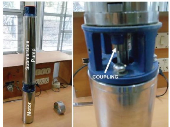
Submersible BLDC motor coupled with the borewell pump
