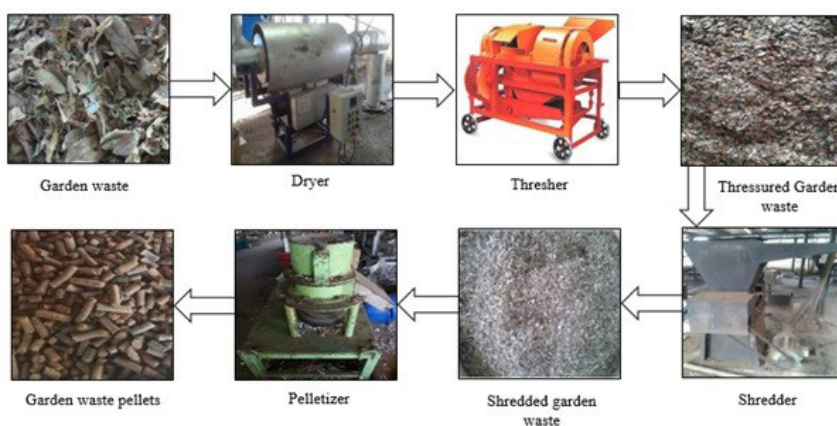
Fig. 1: Processing stages for pelletisation
