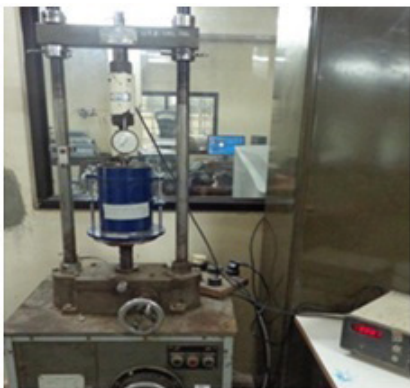
Modified CBR test set up
