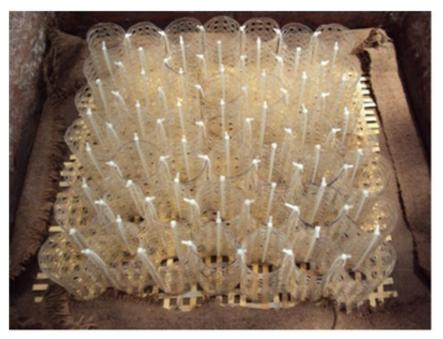
A cellular mattress used in combination with geomaterials is termeda geocell mattress, a three-dimensional (3D) honeycomb structureconsisting of interconnected multiple cells that can be of differentshapes and sizes. Currently, the cells are generally made of strips ofpolymer sheet or geotextile, geogrid sheets, high density polyethylene(HDPE), or Neoloy polymeric
