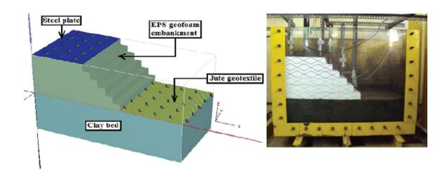
Construction of roadway or railway embankments on soft foundation soil such as marine clay is always a major issue due to poor load carrying capacity and excessive settlements. In such conditions, two major remedies are available. One is ground improvement technique by enhancing the engineering properties of foundation soil and second is reduction in the overburden pressure of structure on foundation soil.
