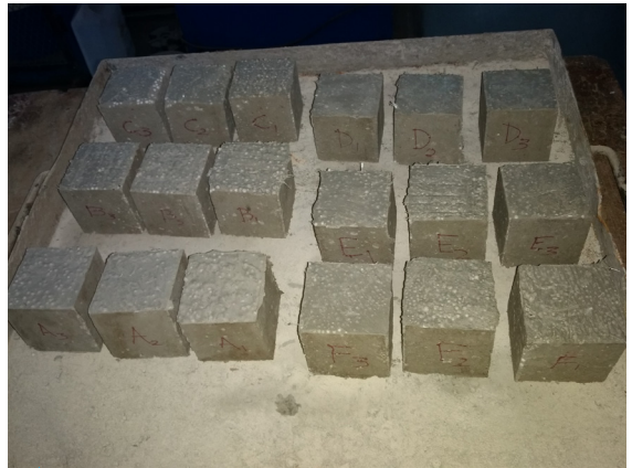
Cube casted using EPS beads and flyash
