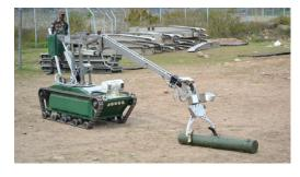
A remotely operated ground vehicle (RoVeR) was designed and developed for use in counter terrorism and counter-insurgency operations by the Indian Army.
