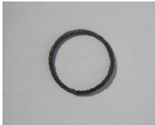
The laser additive manufacturing setup designed and developed at IIT Bombay in action and a 3D printed stainless steel ring
