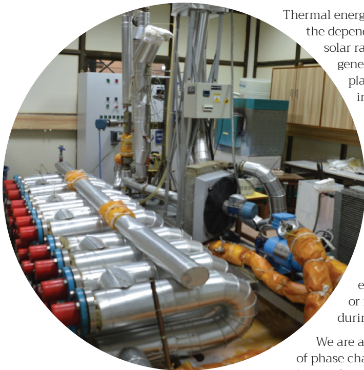
Lab-scale latent heat thermal energy storage at the Thermal Science Lab, Department of Mechanical Engineering
