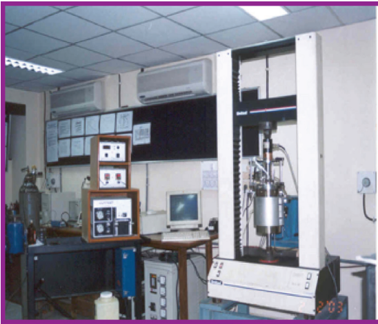
Experimental setup: Study and control of fracture in corrosive environment
