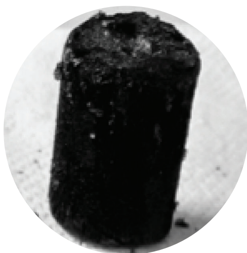
(a) Plug of 3D graphene (b) High resolution scanning electron micrograph showing graphene sheets in the 3D-plug. The central micrograph shows 3D graphene with impregnated silver nanoparticles.
