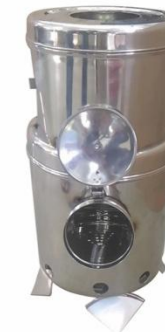
Smokeless stove which produces coal as by-product support from Prof. Sanjay Mahajani, Chemical Engineering
