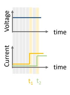
Given a  $t_{pulse} = t_{RNG}$  where P=50%; then 50% devices will be open ("1") and 50% is short ("0"); However, it is impossible to guess, which ones.
