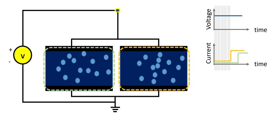
The electrons flowing through the oxide, it disturbs atomic arrangements further; some bonds break stochastically to dislodge atoms permanently to produce defects.
