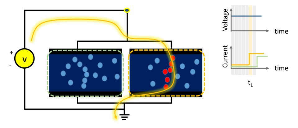
The other MIM devices needs to wait until is defects are generated such that a filament is formed.
