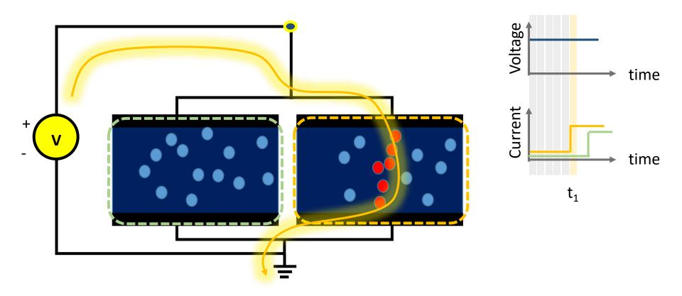
Suddenly, when the filament is formed at time  $t_1$ , the devices shorts and a large current flows; This is the low resistance state or logical "0";
