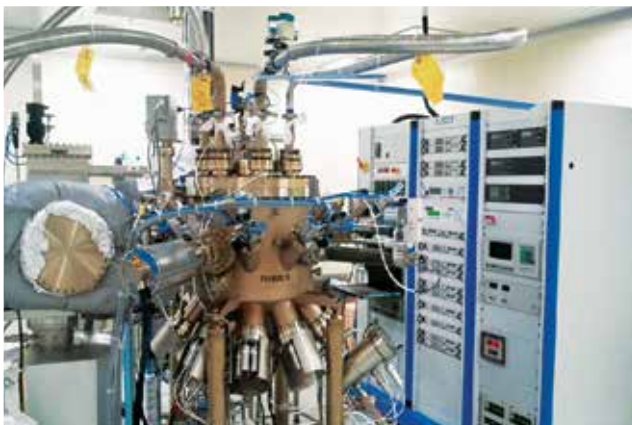
Molecular Beam Epitaxial Growth System
