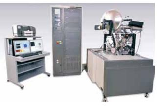
Time-of-Flight Secondary Ion Mass Spectrometer
