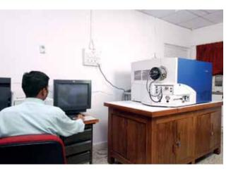
Quadropole Time of flight Tandem mass spectrometer
