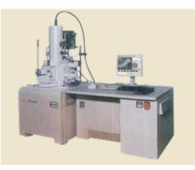
Field emission gun-scanning electron microscope
