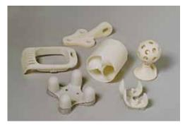
Prototypes made on the FDM Machine
