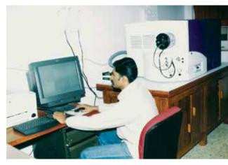
Quadrupole-Time of Flight Tandem Mass Spectrometer
