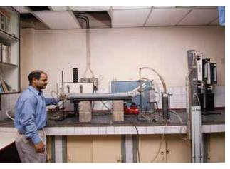
Micro-orifice uniform deposit impacter with diffusion drier
