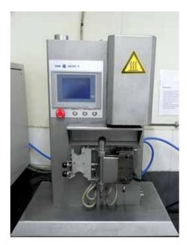
Microcompounder and mini injection moulding
