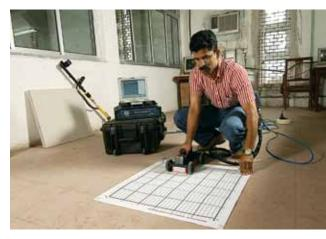
Scanning of RCC slab using Ground Penetrating Radar
