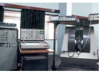
Electron Spin Resonance Spectrometer
