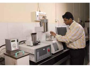
Simultaneous thermal analyzer in the process laboratory
