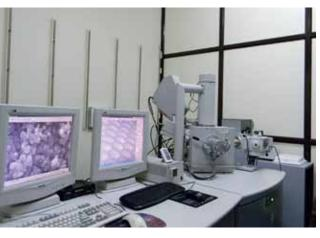
Environmental Scanning Electron Microscope
