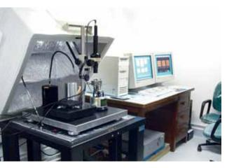
Scanning Probe Microscopy
