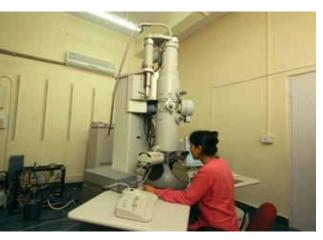
Cryo Transmission Electron Microscope
