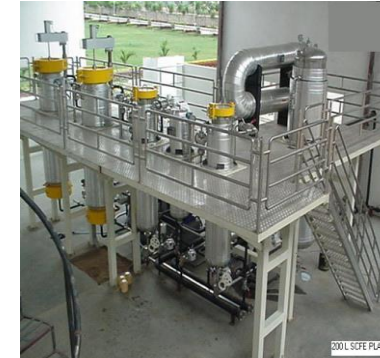
Super Critical Fluid extraction
