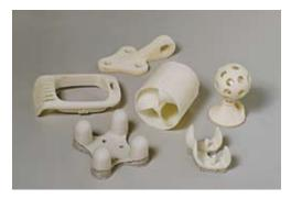
Prototypes made on the FDM Machine
