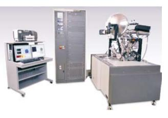
Time-of-Flight Secondary Ion Mass Spectrometer
