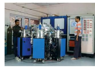
Cluster-tube Hot Wire CVD at the Semiconductor, Thin films and Plasma Processing Laboratory
