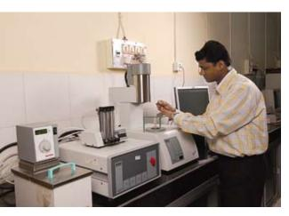
Simultaneous thermal analyzer in the process laboratory
