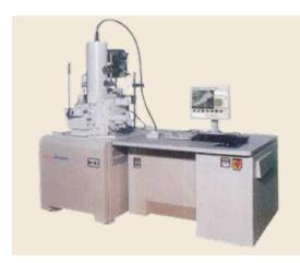
Field emission gun-scanning electron microscope
