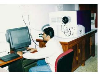
Quadropole-Time of Flight Tandem Mass Spectrometer
