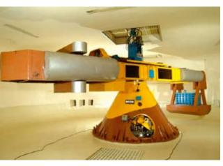
View of a 4.5m radius large beam centrifuge
