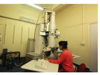
Cryo Transmission Electron Microscope
