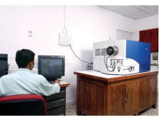
Quadropole Time of flight Tandem mass spectrometer
