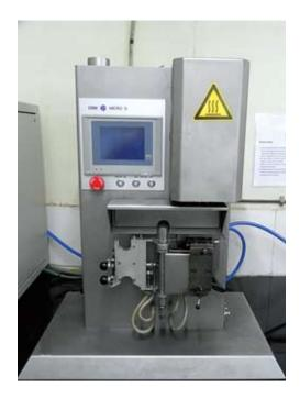
Microcompounder and mini injection moulding
