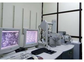
Environmental Scanning Electron Microscope
